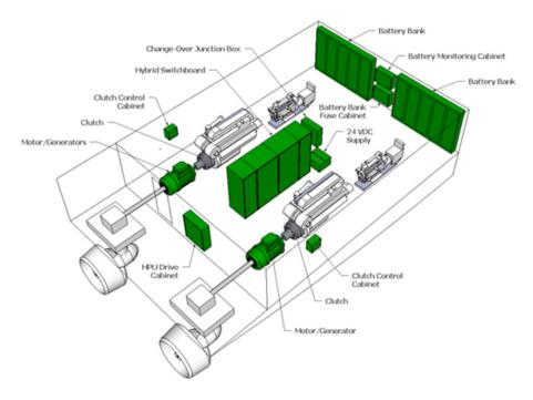
Figure 4.5: Layout of the Foss Tugboat Hybrid System Components
