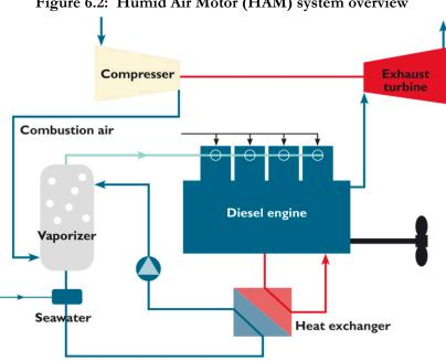
Figure 6.2: Humid Air Motor (HAM) system overview
